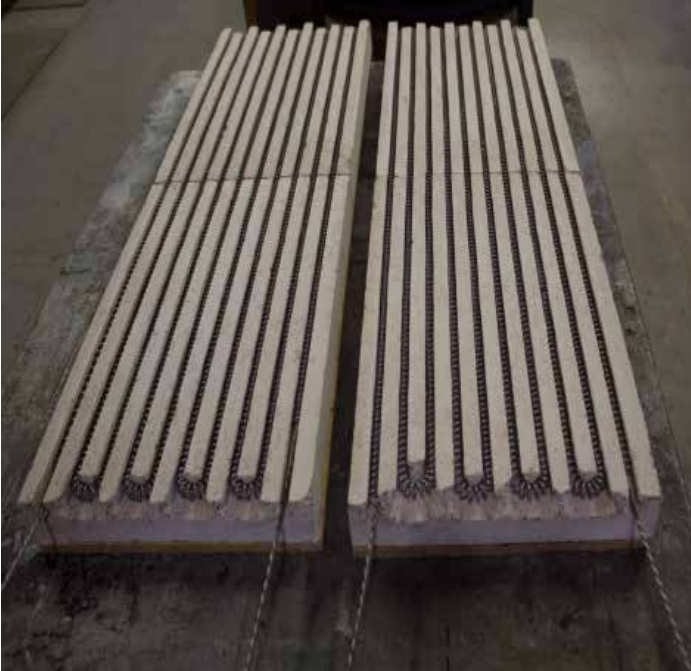
After firing to 1100 °C, the casting is strung with the coiled element wire.
