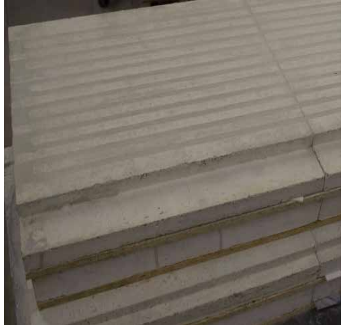
The heaters are finished with element potting compound and ready for installation.
