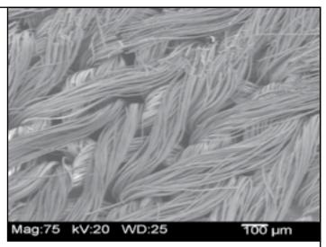
Zirconia Cloth Type ZYK has the unique advantage of being a knit structure. This structure is tied together and irregular shapes can be cut that do not unravel.
