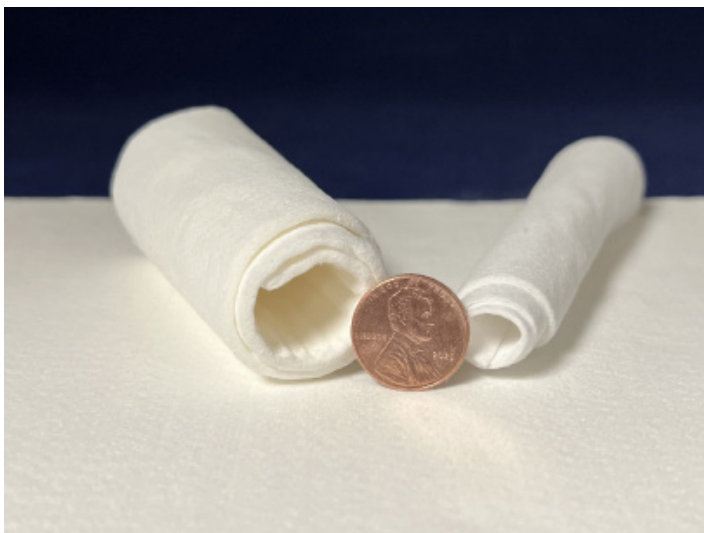
The penny for scale shows the wrappability of ZYF-100 and ZYF-50
