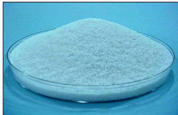
AHB-1 flows freely to a 40° angle of repose
